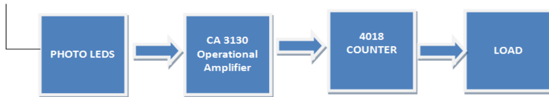
Block Diagram of Infrared Remote Control Switch
